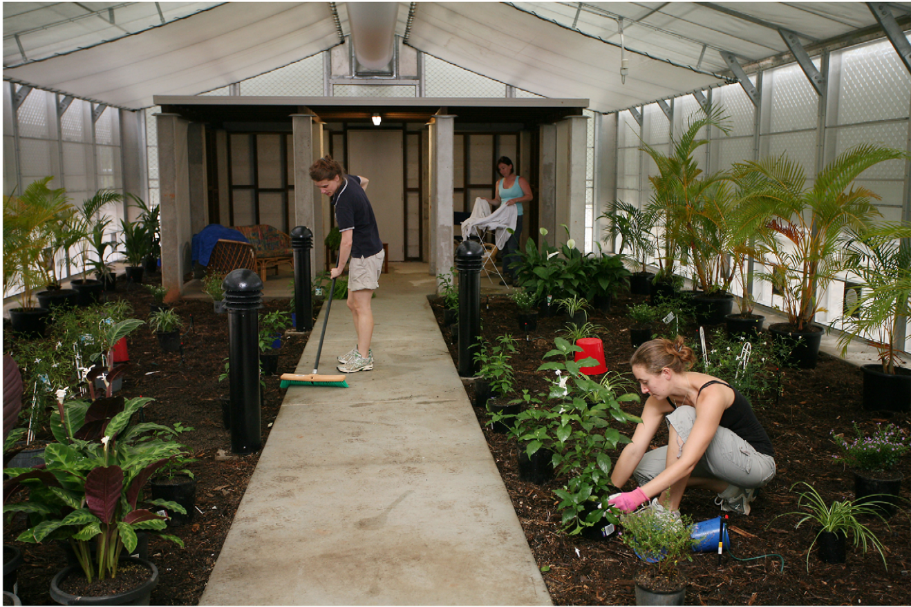
Figure 3. Simulated yard and Queenslander within the MRF SFS. The air distribution sock of the air conditioning system can be seen at the top of the image.
